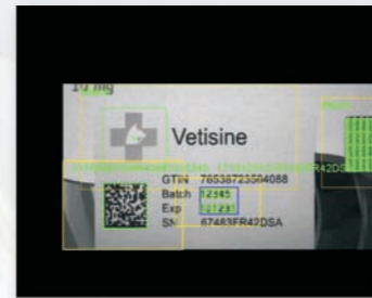
Label alignment inspection, including verification of bar code and human readable text
