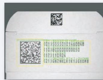
Track & Trace application with verification of GS1-Data Matrix and human readable text consistency (same data content), with additional Data Matrix quality inspection in accordance to ISO 15415
